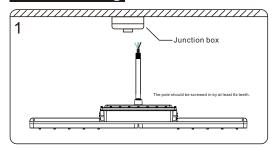
1. Wire the cable through the pole and then install the pole to the fixture.
