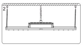
$2.\,\text{Fix}$  the hanging chain to light fixture. Wire the cable through the metal conduit and then connect it with the power.
